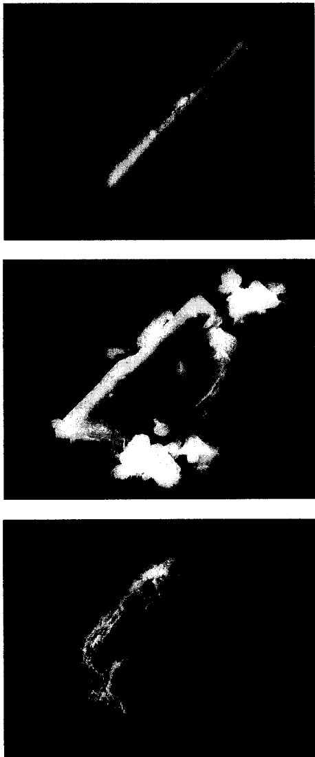
Fig. 1. Scanning electron micrographs of (a) commercial paracetamol; (b) modified paracetamol with Eudragit S 9%; and (c) modified paracetamol with Eudragit S 12%.
